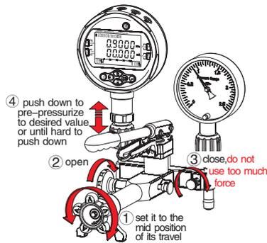
**Pressurizing process and fine adjustment** **D**
